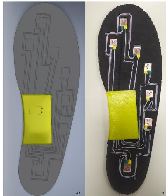
**Figure 5.** (a) 3D design of the insole in AutoDesk Inventor Professional 2018. (b) Inside view of the insole with custom-made capacitive sensors located at the main support plantar points.
