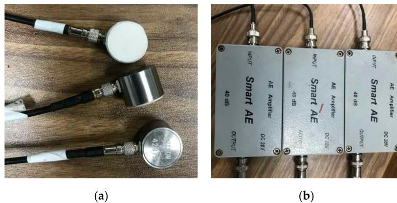
Figure 7. AE sensors and AE amplifiers. (a) AE sensors, (b) AE amplifiers.
