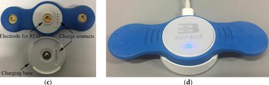
**Figure 4.** (a) The hardware circuit board with lithium-ion battery. (b) Front view of the ECG patch device with disposable ECG electrodes. (c) The three electrodes of the patch and four charge contacts of the patch and the charging base. (RLD = right leg drive). (d) The ECG patch was charging on the charging base.
