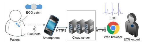
Figure 1. Illustration of the wearable ECG telemonitoring system.
