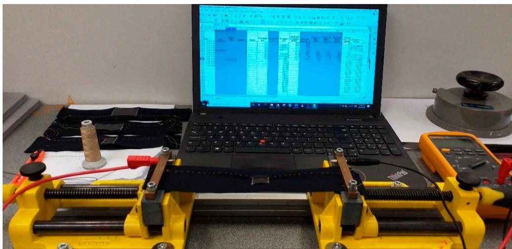
**Figure 5.** Experimental setup for the measurement of resistivity.
