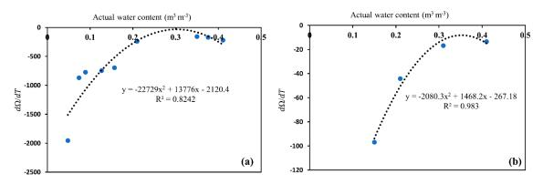
**Figure 8.** Dependence of  $d\Omega/dT$  on water content at (**a**) 0.5 dS/m salinity, and (**b**) 1 dS/m salinity level. The  $d\Omega/dT$  value is the slope of the linear response of sensor resistance to *T* in Figure 6.
