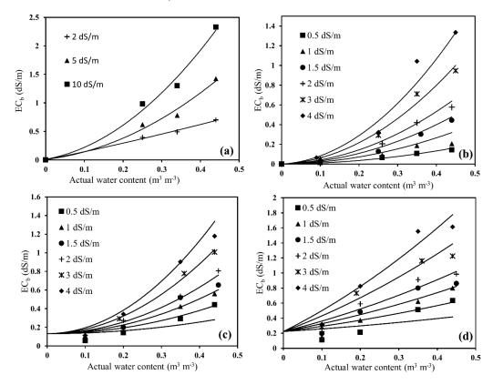
**Figure 5.** Calibration of sensor probe for measuring bulk electrical conductivity ( $EC_b$ ) as a function of water content and salinity in (**a**) glass beads, (**b**) Oso Flaco sand, (**c**) Columbia loam, and (**d**) Yolo clay loam (in Table 5,  $c_1$ ,  $c_2$  and  $c_3$  are optimized parameters for the Rhoades equation [32]). Note that for both glass beads and sand,  $EC_s$  can be assumed to be zero.
