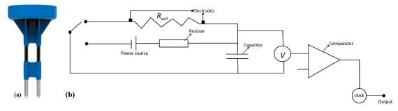
**Figure 1.** (a) The Sensoterra B.V. soil moisture sensor and (b) the circuit diagram of the sensor with resister, capacitor, power source, clock, and comparator.
