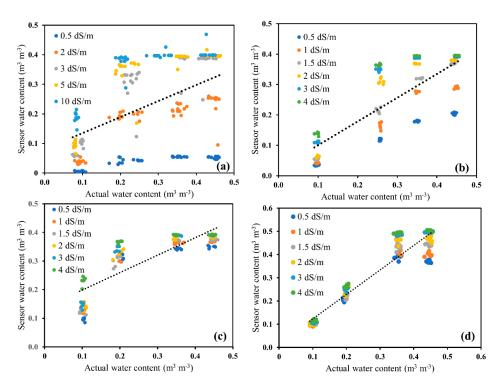
**Figure 4.** Comparison of combined sensor water content with gravimetrically-determined actual water content for (**a**) glass beads, (**b**) Oso Flaco sand, (**c**) Columbia loam, and (**d**) Yolo clay loam over a range of water and electrical conductivity solutions.
