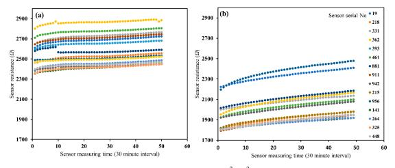
**Figure 2.** Comparison of 15 probes output resistance at  $0.2 \text{ m}^3 \text{ m}^{-3}$  water content with ~1 dS/m solution of electrical conductivity in (**a**) glass beads and (**b**) Oso Flaco sand, over 24 h.
