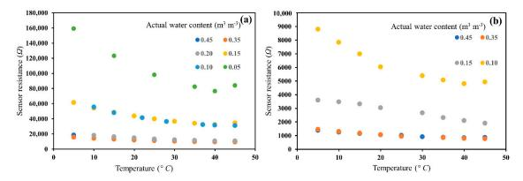
Figure 6. Response of the sensor to temperature at each actual water content and (a) at ~0.5 dS/m salinity, and (b) at 1 dS/m salinity in glass beads. Sensor data represents the raw data in resistance ( $\Omega$ ) at different temperatures.
