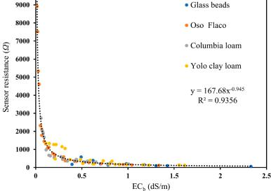
**Figure 7.** Dependence of soil bulk EC on sensor resistance ( $\Omega$ ) for all the four soil types used in this study.
