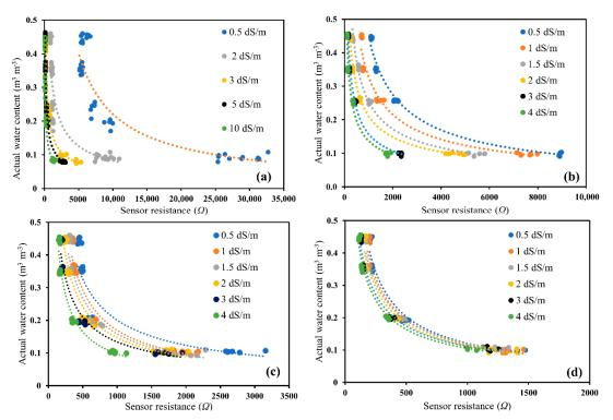
**Figure 3.** Changes in sensor output resistance ( $\Omega$ ) over a range of actual water content (volumetric water content) and solution electrical conductivity ( $EC_w$ ) in (**a**) glass beads, (**b**) Oso Flaco sand, (**c**) Columbia loam, and (**d**) Yolo clay loam.
