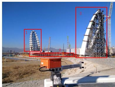
**Figure 11.** Photo of the ArcSAR system and the observed scene.
