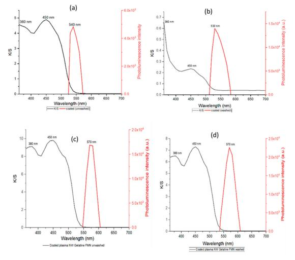
**Figure 7.** Absorbance of FMN gelatin mixture coated on (**a**) untreated PET nonwoven coated, unwashed sample (**b**) untreated PET nonwoven coated, washed sample (**c**) plasma-treated PET nonwoven coated, unwashed sample (**d**) plasma-treated PET nonwoven coated, washed sample.
