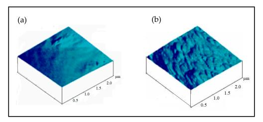
**Figure 3.** Atomic force microscopy (AFM) images of (**a**) untreated PET, (**b**) ATMP-treated fiber surface of nonwovens.
