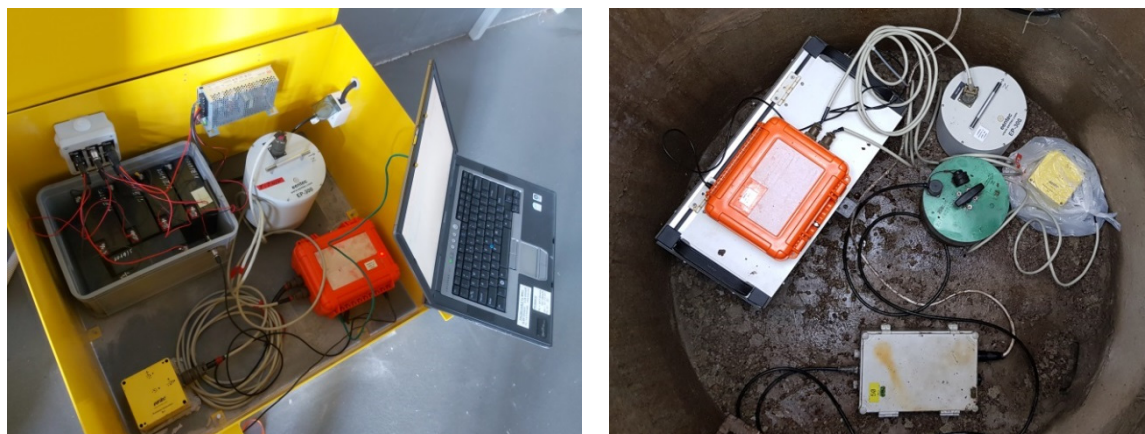
Figure 4. Systems for 6-DoF measurement installed near the Rudna-I shaft (left) and at the Zelazny Most tailing pond (right).
