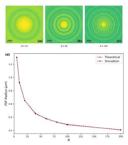
**Figure 3.** (**a**–**c**) False color images of simulated Point Spread Function (PSF) on a logarithmic scale, when the number of zones *N* equals to 10, 40, and 100. (**d**) Theoretical and simulated PSF spot radius versus N.
