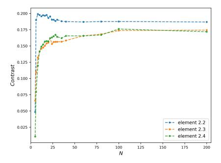
**Figure 7.** Contrast plots of different width bars versus number of zones *N*:the images are simulated under the same conditions of Figure 4, the studied bars of test chart are shown in Figure 4f.
