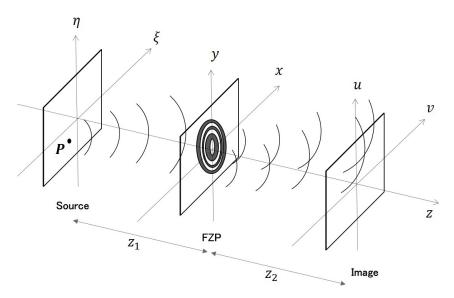
**Figure 1.** Generalized schematic of Fresnel Zone Plate (FZP) optical system: the point source *P* on the plane  $(\xi, \eta)$  emitting a spherical wave is intercepted and diffracted by the FZP on the plane (x, y). The image of the source is formed on the plane (u, v).  $z_1$  and  $z_2$  represent respectively the source–FZP distance and the FZP–image distance.
