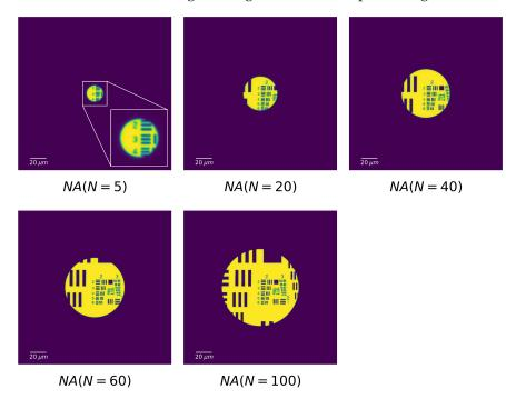
**Figure 8.** False color numerical images of the USAF 1951 test target imaged by refractive lens. The NA of the refractive lens equals to the NA of the FZP when the number of zones of FZP is 5, 20, 40, 60, and 100. Each image dimension is  $200 \times 200 \ \mu\text{m}^2$ .
