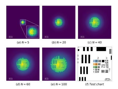
**Figure 5.** (**a**–**e**) False color numerical images of the USAF 1951 test target imaged by FZP with different number of zones. The object—FZP distance is 3f and the FZP–image distance is 1.5f. Each image dimension is  $200 \times 200 \ \mu\text{m}^2$ . (**f**) Zoomed part of interest on the test chart: for the following part, the blue, orange and green colored elements of bars in group 2 are respectively noted as elements 2.2, 2.3, and 2.4.
