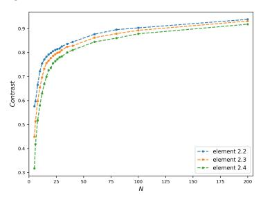
**Figure 9.** Contrast plots measured from the images formed by refractive lens: For the sake of clarity, the horizontal axis displays the number of zones of the FZP having the same NA than the refractive lens. Moreover, the images are simulated under the same conditions as for Figure 5.
