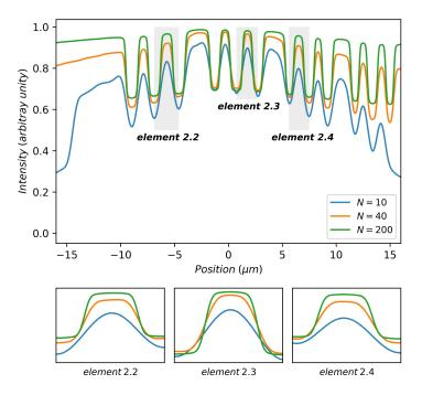
**Figure 6.** Intensity profile plots of images in focus with various numbers of zones: the images are simulated under the same conditions of Figure 4. Three zoomed parts of plot corresponding to different groups of bars are given below the main plot.
