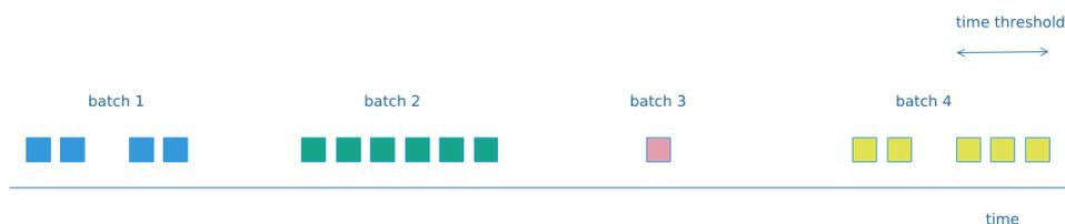
Figure 6. Building packet batches for Non-IP protocols.
