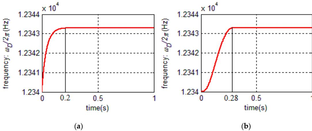
Figure 16. (a) Step response of the PLL linearized model and (b) step response of the PLL original model.
