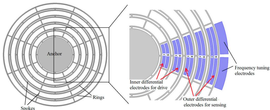
Figure 1. Diagrammatic sketch of MEMS disk resonator.
