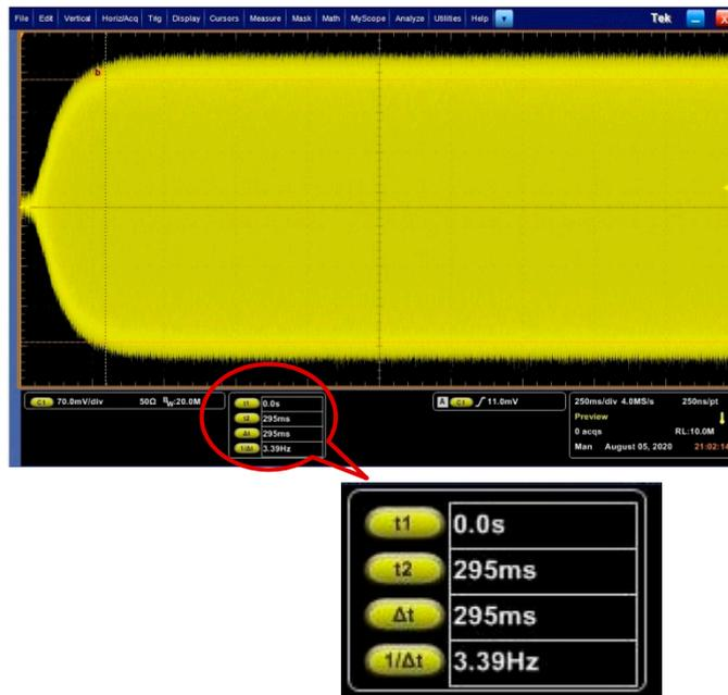
Figure 17. Start-up waveform of PLL loop with DRG experimental board.
