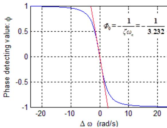
Figure 13. Relationship curve between  $\Phi$  and  $\Delta\omega$ .
