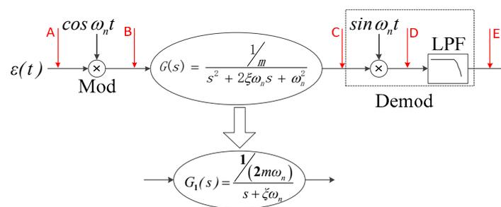
**Figure 6.** The modules <modulator–gyroscope–demodulator> in series and their equivalent first-order transfer function.
