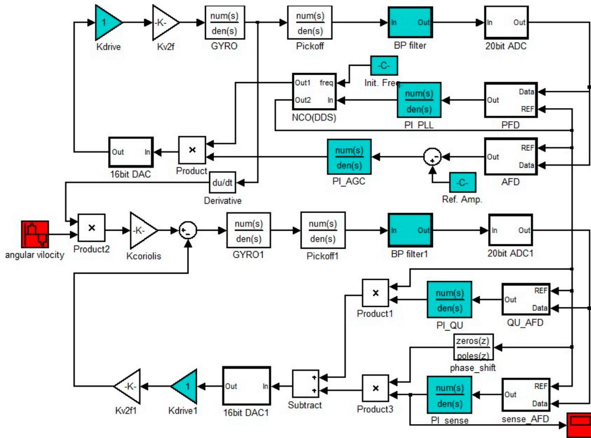
Figure 3. Original mechatronics model for DRG with a configurable ASIC.
