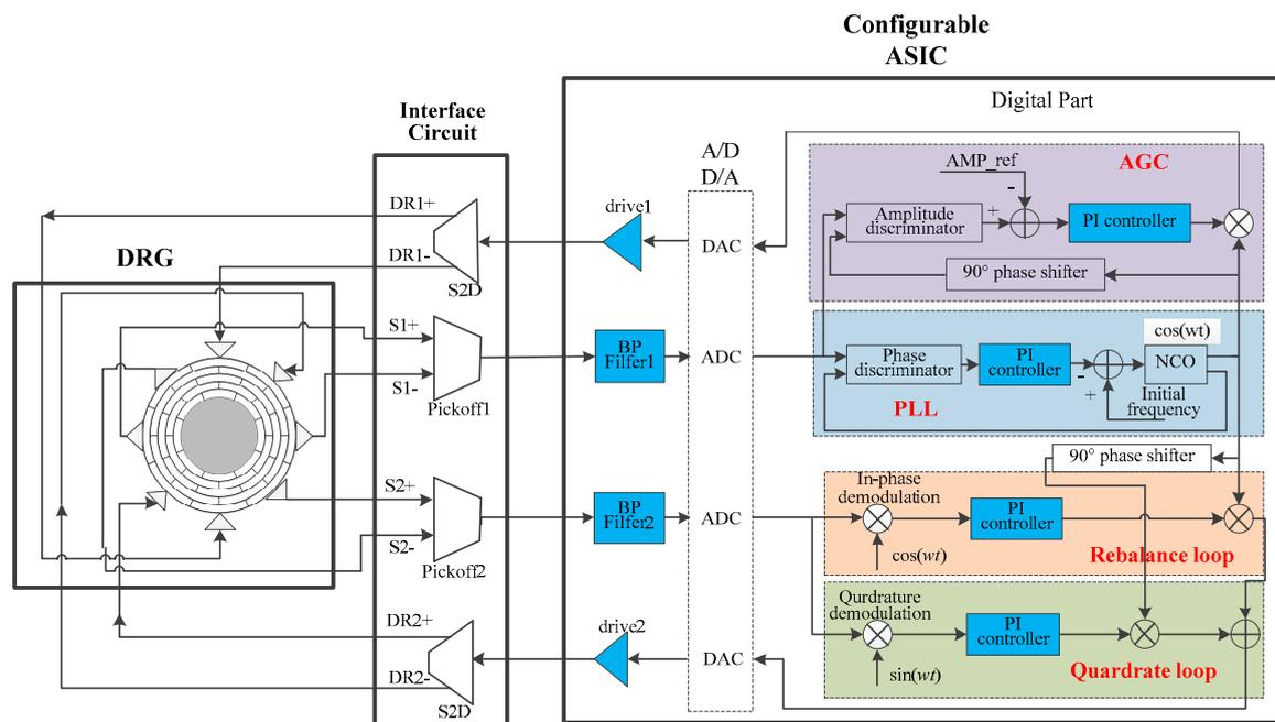
**Figure 2.** Closed-loop system constituted by the MEMS disk resonator and a configurable ASIC.
