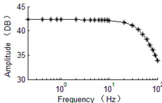
Figure 20. Amplitude–frequency characteristic curve of the original model.
