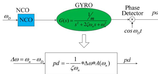
**Figure 14.** The models < oscillator–gyroscope–phase detector > in series are approximated as a gain term.
