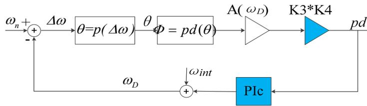
Figure 12. Order-reduction model of PLL.
