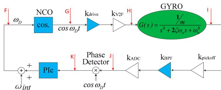
Figure 11. PLL loop after using equivalent gain method.
