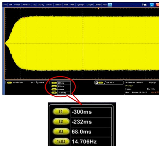
**Figure 10.** Start-up waveform of AGC loop with DRG experimental board.
