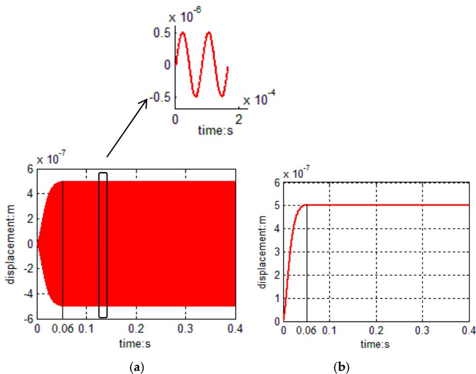
Figure 8. (a) Step response of AGC original model and (b) step response of the AGC linearized model.
