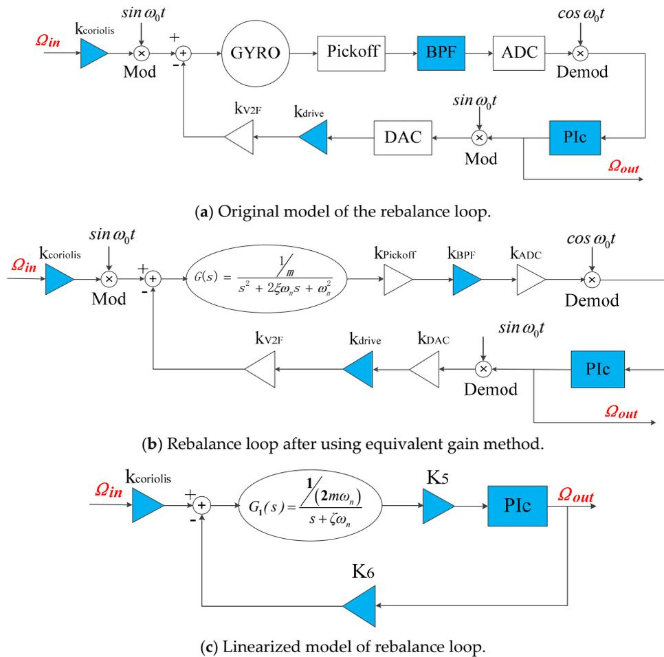
Figure 18. Linearization process of the rebalance loop.
