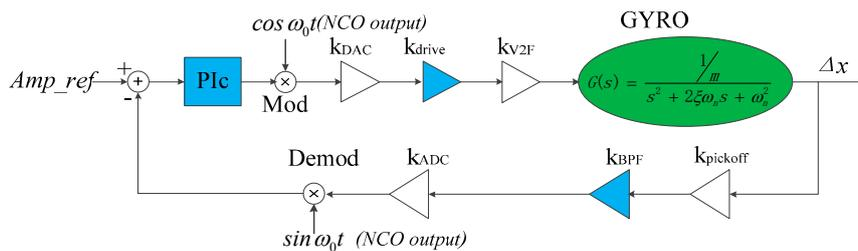
(a) Closed-loop AGC with some function parts replaced by gain terms.
