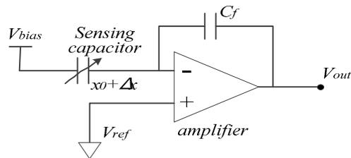
Figure 4. C/V circuit implemented by a charge amplifier.
