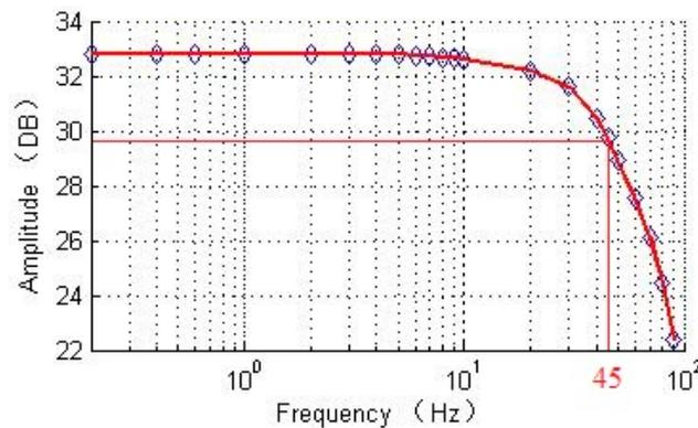
**Figure 21.** Tested bandwidth of DRG experimental board.
