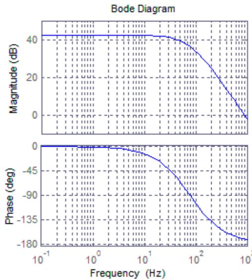
Figure 19. Bode diagram of the rebalance loop’s linearized model.
