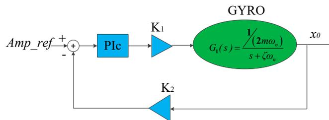
Figure 7. Order-reduction model for AGC loop.
