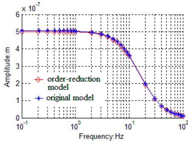
**Figure 9.** Frequency response characteristics of AGC loop based on the linearized model and the original model.
