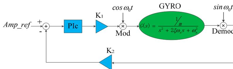
(b) Closed-loop AGC with gain terms merged and locations exchanged.
