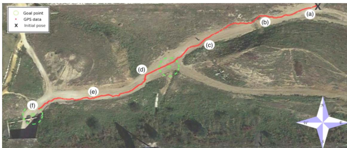
**Figure 13.** GPS measurements during autonomous navigation on the hollow. Locations where each photograph of Figure 12 was taken are indicated.
