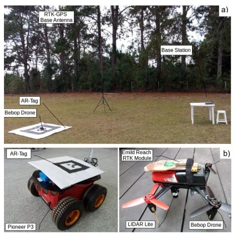
**Figure 2.** Architecture components. (a) Inspection site: base station, RTK-GPS, and UAV. (b) Detail of the Bebop drone with RTK-GPS module and Pioneer P3 with the augmented reality tag (AR-Tag).
