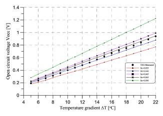
**Figure 9.** Comparison of different model adjustments and the acquired data from the TEG used in the prototype.
