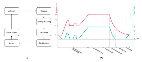
Figure 1. (a) Instrument life-cycle process diagram, (b) steam sterilization overview.
