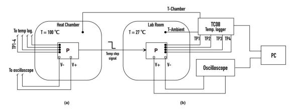
**Figure 5.** Scheme of the conducted experiment with the prototype (P). Measurement setup used in the heat chamber (a) and while simulating temperature step signal in the laboratory room (b).
