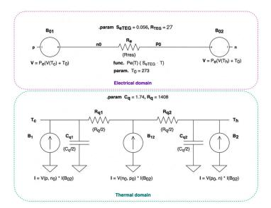
**Figure 4.** Kubov's thermo-electrical generators (TEG) electric circuit representation with SPICE directives. The upper part is a model of electrical domain of the TEG while the bottom part models the thermal behavior of the TEG.
