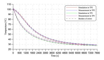
**Figure 7.** Comparison between simulated results and thermal measurements using K-Type thermocouple in test-points TP1 and TP2.
