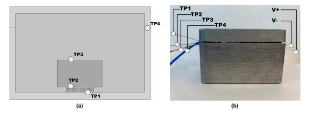
**Figure 6.** Test points of the model (**a**) and prototype (**b**) to compare the heat distribution in a simulated environment in comparison to the prototype tests in the heat chamber.
