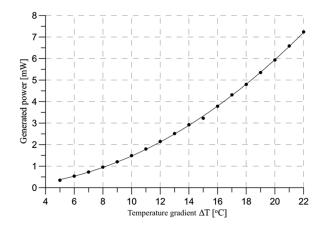
Figure 10. Power generated on the different thermal gradients with matched load.
