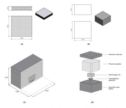
**Figure 3.** (a) A thermoelectric generator with its dimensions used for this study, (b) a steel heat storage unit (HSU), (c) cross-section of the prototype and 3D module with the outer sizes, (d) exploded view of used 3D model as well as a prototyped module. All the sizes are in mm.
