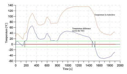
**Figure 8.** Temperature inside the autoclave and on the surface of the walls of the prototype (orange line) during single steam sterilization procedure, and corresponding thermal gradient across the TEG module inside the prototype (blue line).
