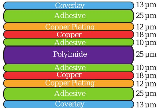
**Figure 7.** Stack-up used during fabrication. Additional top and bottom polyamide layers were added for sensor protection and isolation.
