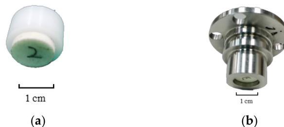
**Figure 4.** Home-made air-coupled transducer (a) without pre-tightening; (b) with pre-tightening.
