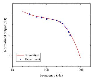
**Figure 3.** Normalized PT signal as a function of pump modulation frequency. The red line is calculated by COMSOL Multiphysics and the blue dots are the experimental data. Error bars show the standard deviation (s.d.) of measured data.
