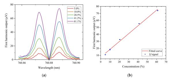
**Figure 6.** (a) First harmonic output signal for 5%, 10%, 20.5%, 41.2% and 61.1% oxygen in nitrogen. (b) Peak value of the PT signal as a function of oxygen concentration from 5% to 60%. Error bars show the s.d. of the PT signal.
