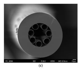
**Figure 2.** (a) Absorption lines of oxygen from 759.5 to 762 nm at 293 K and 1 atm determined by the HITRAN database. (b) Spectral transmission of the HC-NCF. (c) The cross-sectional image of the HC-NCF.
