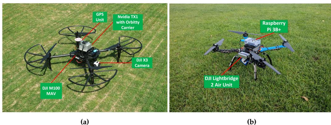
**Figure 1.** The UAV platforms; DJI M100 (a) and the custom quadcopter (b).
