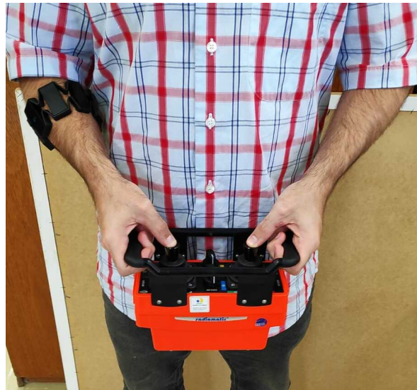
Figure 11. Robot controls. There is a fusion between data from an industrial joystick and a Myo armband to control the robot.
