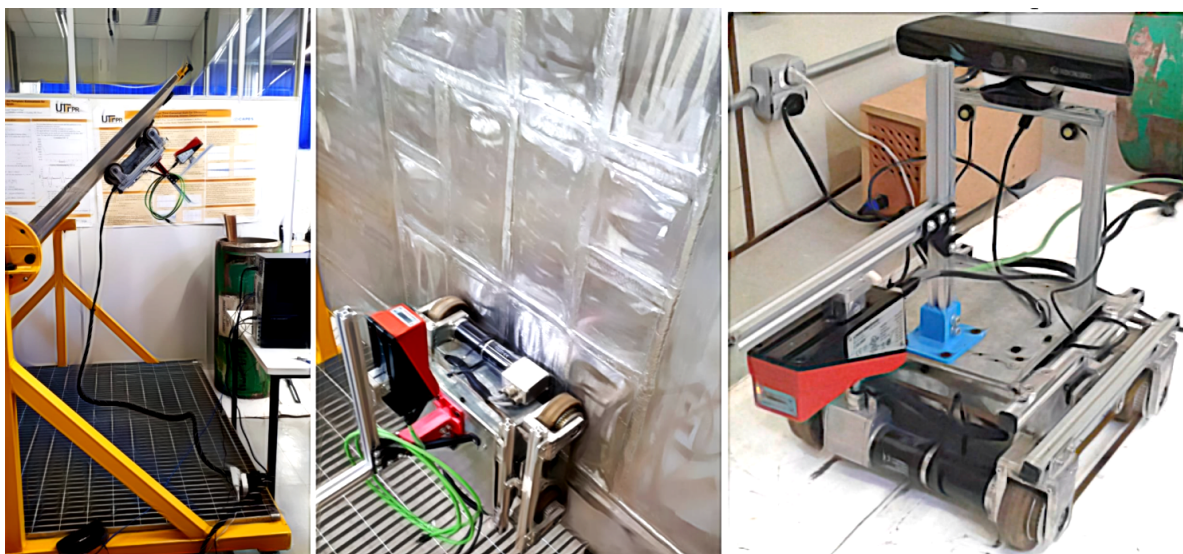
Figure 2. Autonomous Inspection Robot 1 (AIR1). A robot conceived/developed to inspect weld beads in storage tanks containing liquefied petroleum gas. A profile sensor, facing downwards, is positioned in front of the robot.
