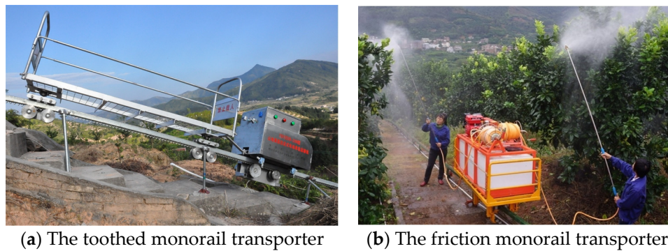
Figure 1. Two types of mountainous monorail transporters.
