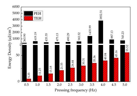
**Figure 13.** Energy densities of PEH and TEH under the variable pressing frequency of 0.5–5 Hz and at a 4 mm gap width.
