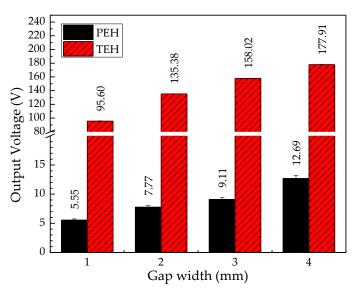
Figure 11. Output voltage of PEH and TEH.
