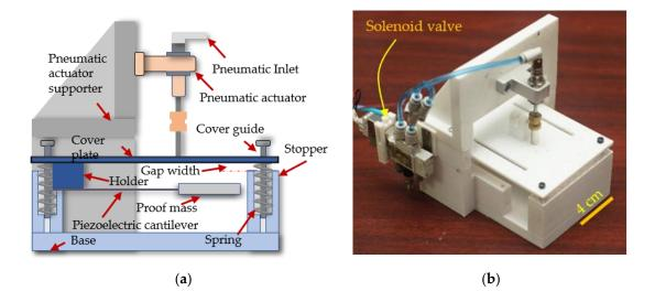
**Figure 1.** Piezoelectric energy harvester (PEH) test bench: (**a**) cross-section of PEH; (**b**) photograph of PEH test bench.
