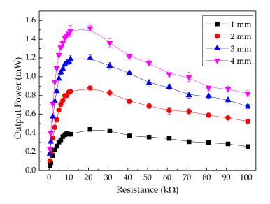
Figure 9. Output power of TEH test bench at various gap widths from 1 mm to 4 mm.
