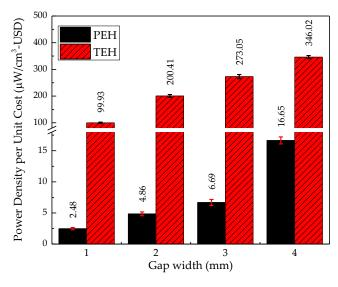
Figure 14. Power density per unit cost of PEH and TEH at a 4 mm gap width.
