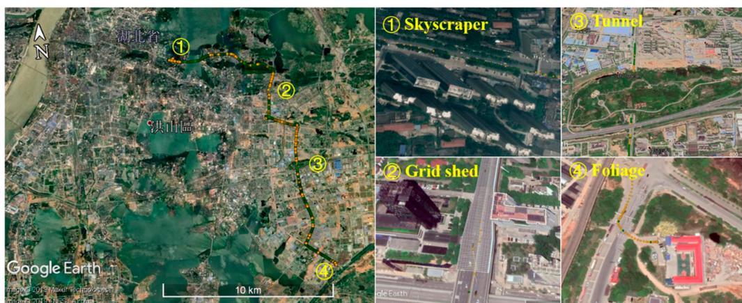
**Figure 11.** Trajectory and four typical GNSS challenging environments of test #2.
