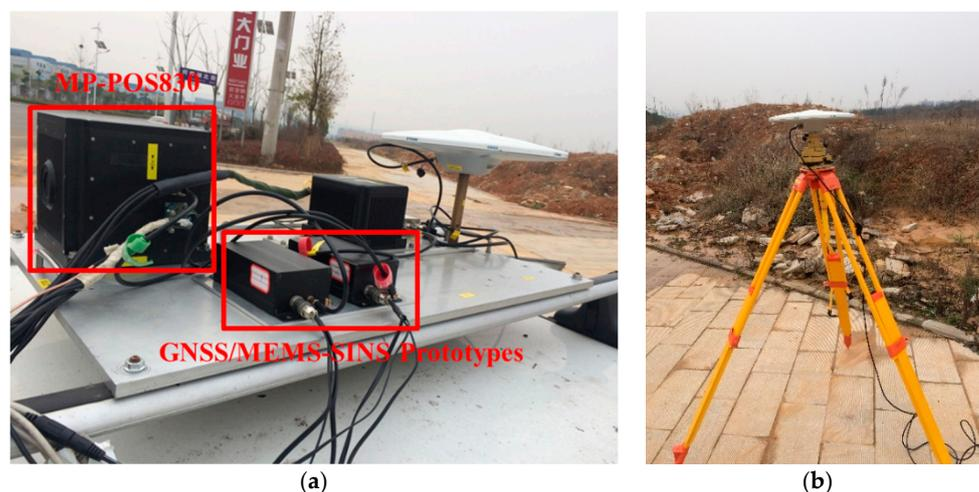
Figure 4. Test setup. (a) Equipment mounted on the roof of a car; (b) Base station.
