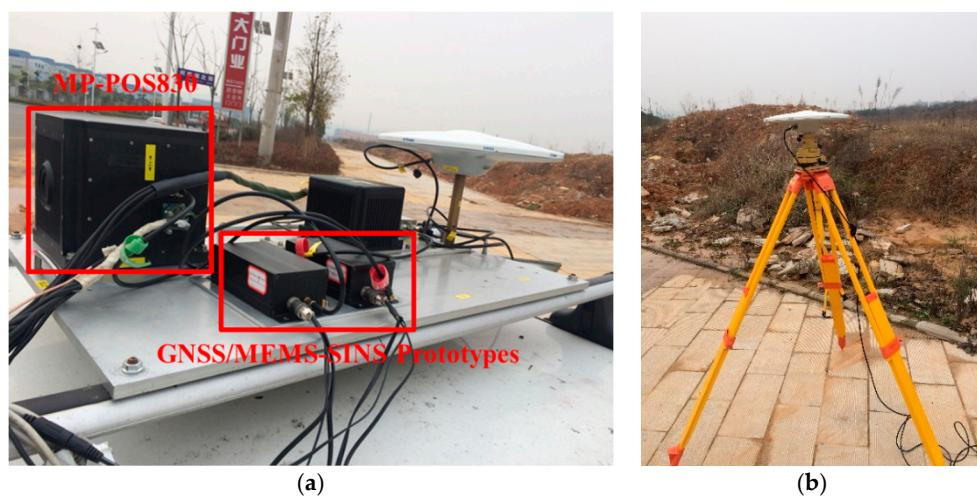
**Figure 4.** Test setup. (a) Equipment mounted on the roof of a car; (b) Base station.
