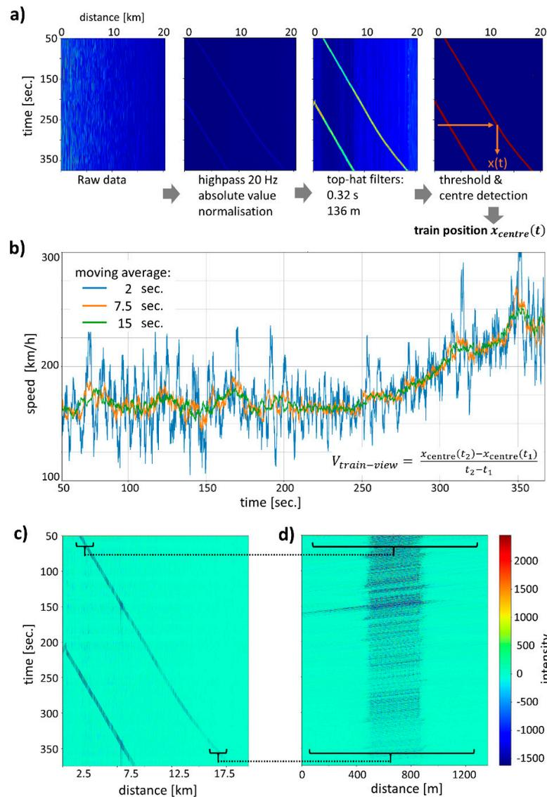
**Figure 2.** (a) The train position  $x_{center}(t)$  as a function of time is determined by applying the shown filtering. (b) From this position, the train velocity of the ICE 4 train can be calculated at each given moment in time. (c) Using the previously determined position of the train, a section of DAS data with the train in the center can be cut and arranged to arrive at the ‘train-view’ representation of the data in (d).
