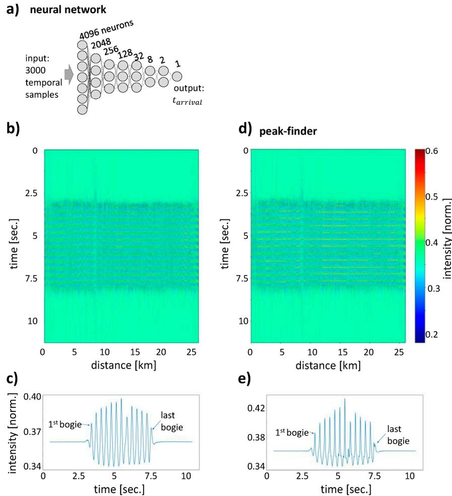
**Figure 4.** (a) Artificial neural networks (ANN) can successfully predict the precise arrival times of a bogie cluster so that a well aligned rail-view graph (b) can be generated. (c) Taking the spatial average of the rail-view graph, all bogie clusters can clearly be resolved as 13 peaks. A peak finder algorithm performs similarly to the ANN in aligning the bins for a rail-view graph (d) and again 13 peaks can be found as well but the peak height is more uneven (e).
