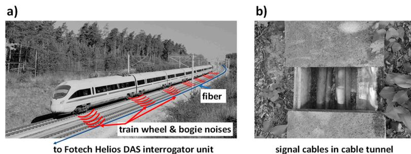
**Figure 1.** (a) Schematic of ICE train on ballastless track emitting noises that are picked up by a fiber optic distributed acoustic sensing (DAS) interrogator. (b) Standard telecom signal cables lying within cable tunnels are used for sensing.
