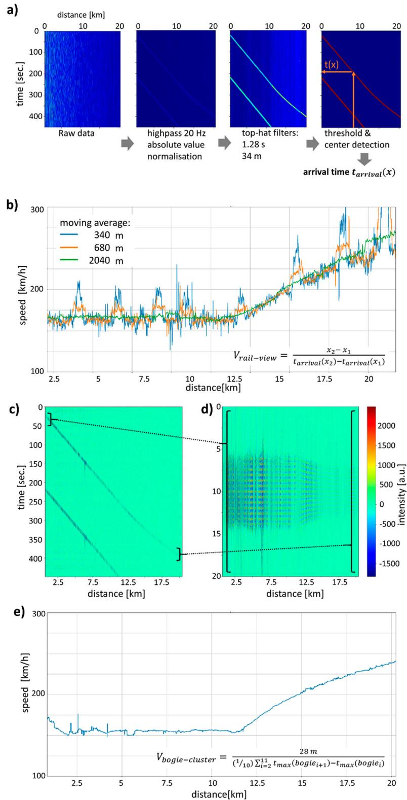
**Figure 3.** ‘Rail-view’ analysis of the DAS data at fixed positions as a function of time. **(a)** Filtering and center detection are similar to Figure 2a, however, the train arrival time  $t_{arrival}(x)$  is determined here. **(b)** From the rail-view data, the train speed is calculated and shown for different averaging lengths. Peaks in the velocity are due to fiber loops. **(c,d)** Arranging the 20 Hz filtered data in **(c)** such that the
