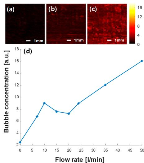
**Figure 8.** 2D ultrasound images of the liquid flowing in the pipe (color bar represents the ultrasound signal strength) at flow rates of (a) no flow, (b) 25 L/min, (c) 50 L/min, and (d) the relative bubble concentrations at varying flow rates.
