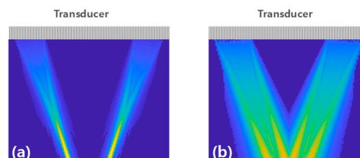
**Figure 2.** Transmitted ultrasound beam profiles of the (a) focused beam and (b) plane wave in the liquid. An array transducer was on top of the pipe.
