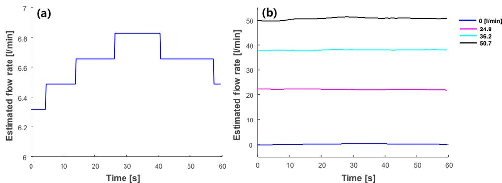
**Figure 7.** Estimated flows for (a) no flow, and (b) eight flow rates (reference flows at 0, 24.8, 36.2, and 50.7 L/min) after zero-flow calibration.
