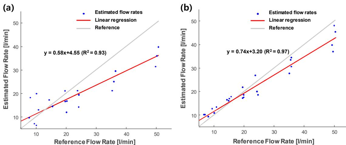
**Figure 6.** Estimated flow rates using (a) focused beam and (b) plane waves.
