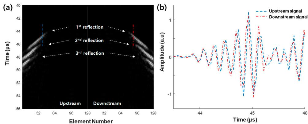
**Figure 5.** Ultrasonic (a) 2D images and (b) signals of upstream (blue dashed line) and downstream (red dash-dotted line) at a flow rate of 35 L/min. Dashed and dash-dotted lines in (a) are the positions where the ultrasonic signals in (b) are displayed. The arrows indicate the 1st, 2nd, and 3rd reflections.
