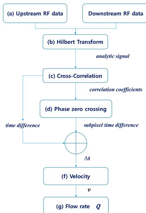
Figure 4. Flow estimation block diagram.
