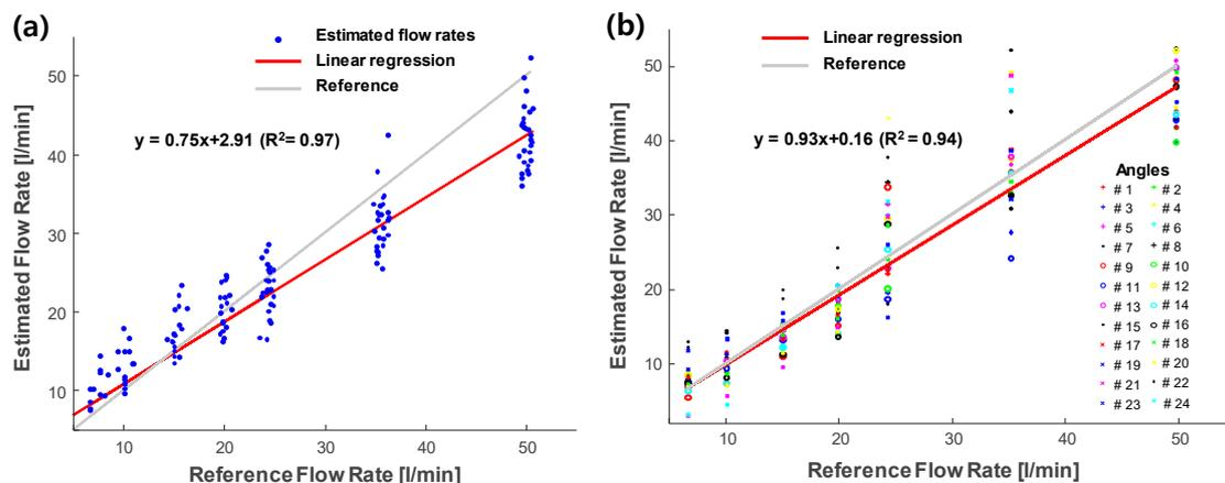
Figure 10. Estimated flow rates using (a) a single plane wave and (b) multiple angular compensation.
