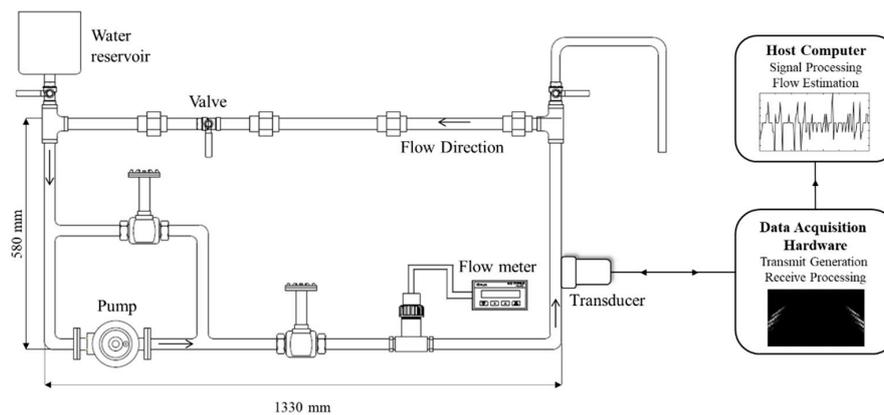
**Figure 1.** Experimental setup for liquid flow in the pipe system and ultrasound data acquisition system with array transducer.
