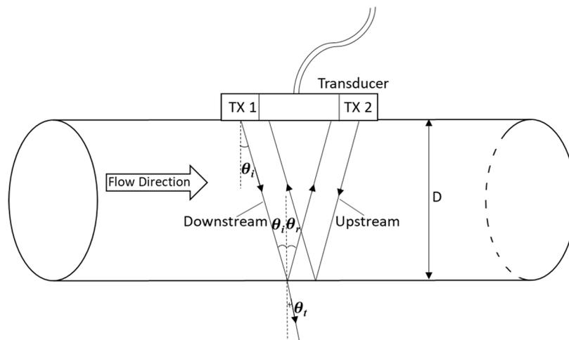
**Figure 3.** Illustration of pipe geometry and propagation and reflection of ultrasound waves.
