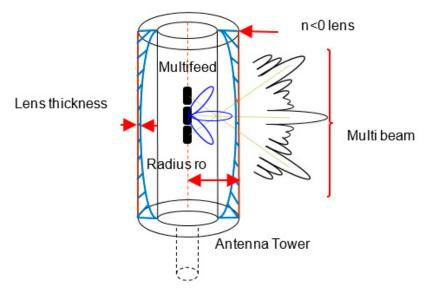
Figure 1. Proposed mobile base station structure.
