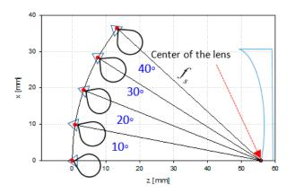
Figure 19. Feed position arrangement.
