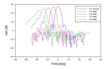
**Figure 20.** Antenna gain for scanning angle  $0^{\circ}$  to  $40^{\circ}$ .
