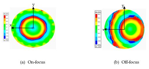
Figure 23. Electric phase distribution.
