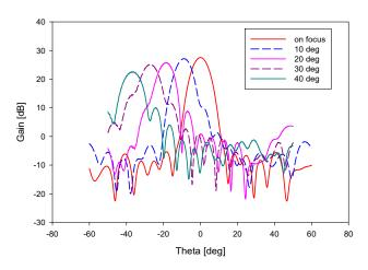
**Figure 15.** Antenna gain for scanning angle  $0^{\circ}$  to  $40^{\circ}$ .
