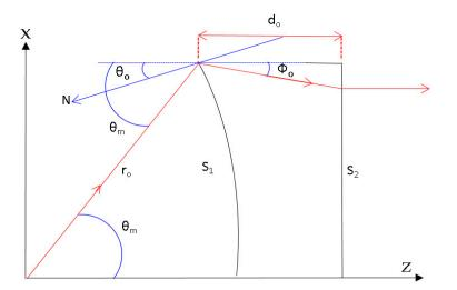
Figure 5. Initial parameters at the lens edge.
