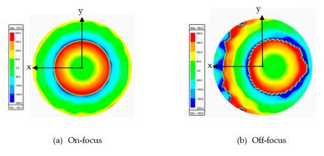
Figure 17. Electric phase distribution.
