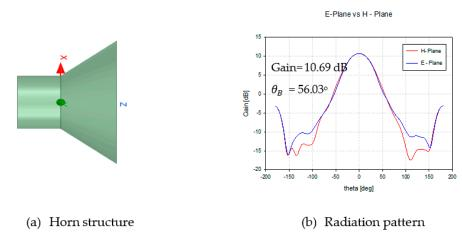
Figure 12. Performance of horn antenna as a feed radiator.
