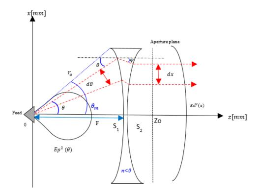
Figure 2. Lens configuration and parameters. Table 1. Antenna parameters.
