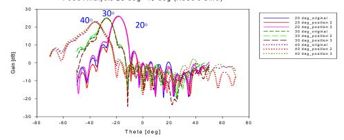
Figure 27. Antenna gain for all feed position for Abbe's sine lens.
