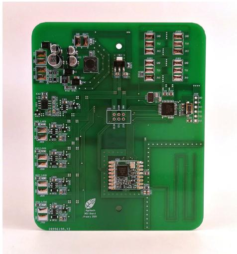
(a) On the left side are placed the solar powered battery charger circuit, the square signal generator and 4 peak detector circuits. On the right side, a LDO voltage regulator, the low-power MCU and the LoRa module.
