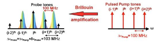
**Figure 16.** SBS interaction between a multi-tone pump wave and a multi-tone probe wave as done in the frequency-sweep free method [63].
