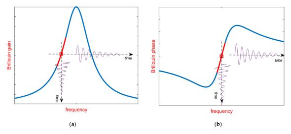
**Figure 5.** Principle of operation of the SA-BOTDA method: the strain-induced spectral shifts of the BGS (**a**) or the BPS (**b**) can be regarded as temporal variations of the probe frequency around its working point.
