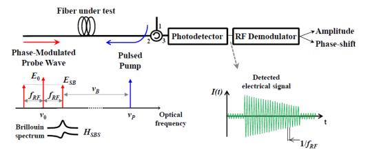
**Figure 10.** SBS interaction between a pulsed pump and a phase-modulated probe wave for dynamic strain measurements [47].
