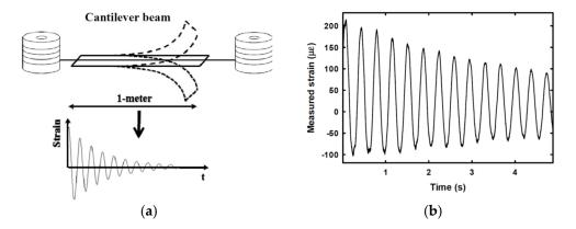
**Figure 11.** Experimental demonstration of dynamic strain measurement (**b**) over a 1-m cantilever beam subjected to vibration (**a**), carried out using the setup of Figure 10 [47].
