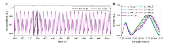
**Figure 24.** (a) Transmitted probe power as a function of time, showing a sequence of BGSs impressed on it due to interaction with the pump pulse. (b) Zoomed view of the portion of the probe signal corresponding to the segment of the fiber subjected to strain. The waveform has been acquired with an averaging factor of 200 and a pump pulse duration of 10 ns and an OCC duration of 20 ns [70].
