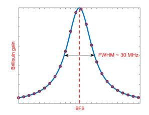
**Figure 1.** Brillouin Gain Spectrum in a conventional silica fiber. The red circles represent the frequencies acquired for BFS extraction.
