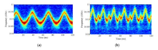
**Figure 22.** BGS acquired using the fast BOTDA method combined with the differential pulse-pair technique [68]. The vibrating fiber was excited at a frequency of (**a**) 33.3 Hz or (**b**) 50 Hz.
