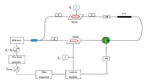
**Figure 3.** Experimental setup employed for BOCDA measurements; EOM, electro-optic modulator; PD, photodiode; FUT, fiber under test (Adapted from Ref. [39]).
