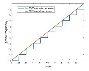
**Figure 20.** Probe frequency sweep used for stepped sweep [67] and linear sweep [69] BOTDA measurements. *T* represents the time slot allocated for the acquisition of each Brillouin gain profile (in the ideal case, e.g., no averaging, *T* corresponds to the roundtrip time of the pump pulse over the fiber length).
