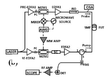
Figure 17. Experimental setup employed for sweep-free BOTDA measurements [63].
