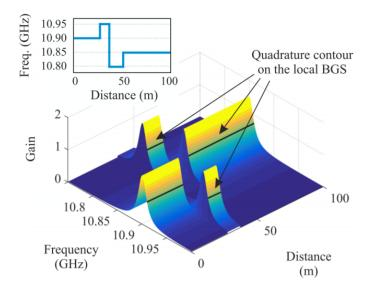
**Figure 8.** Fast changing the probe frequency allows the latter to lie within the slope of each local BGS, even in case of spatial nonuniformities [55].
