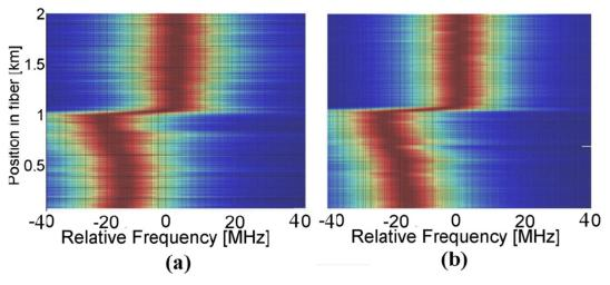
**Figure 18.** Measurement of the BGS along a 2-km FUT using (**a**) the frequency-sweep method, with 30 frequency tones spanning 90 MHz, reconstructed at a spatial resolution of 50 m; or (**b**) Using a classical BOTDA with 3MHz sweeping step [63].
