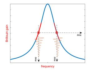
**Figure 14.** In the dual slope-assisted BOTDA method, the probe frequency is switched between the two slopes, while the dynamic strain is extracted from the ratio between the signals acquired from the two slopes [61].
