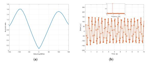
**Figure 13.** (a) Amplitude of the heterodyne signal normalized to its dc value, computed for a pulse duration of 10 ns, as a function of detuning from resonance (b) Dynamic strain measured on a 1-m long cantilever beam subjected to vibration. (The inset shows the FFT of the acquired waveform [60]).
