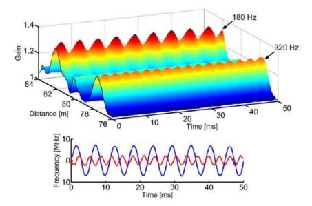
**Figure 9.** (**Top**) Brillouin gain variations acquired along an 85-m long fiber with two sections subjected to dynamic strain. (**Bottom**) Corresponding BFS changes in the two positions [55].
