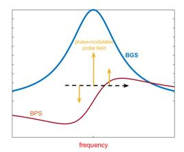
**Figure 12.** Schematic representation of the interactions involved in the heterodyne slope-assisted method [60]. The BGS and BPS affect both the carrier and the two first-order sidebands of the phase-modulated probe, leading to the appearance of an RF beat note on the transmitted probe intensity.
