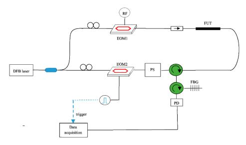
**Figure 2.** Conventional BOTDA configuration. PS: polarization scrambler; FBG: fiber Bragg grating. EOM: Electro-optic modulator. PD: photodetector.
