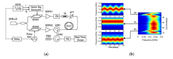
**Figure 19.** (a) Experimental setup for fast frequency sweeping BOTDA; (b) BGS acquired in one fixed and two vibrating locations of the FUT [67].
