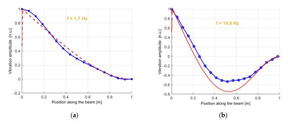
**Figure 7.** Dynamic strain amplitude related to the (**a**) first and (**b**) second mode of the cantilever beam. Mode frequencies are 1.7 Hz are 10.8 Hz, respectively. The blue lines represent the mode shapes measured using the SA-BOTDA method, while the red lines represent the FEM result [52].
