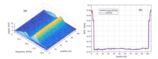
**Figure 21.** (a) BGS acquired by using a linearly swept probe frequency, in a sweep time of 33 ms; (b) Comparison of the BFS profile acquired using either the FAST BOTDA method with a linearly swept frequency, or the conventional BOTDA method.
