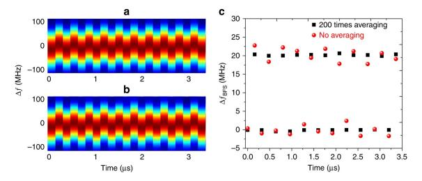
shows the time evolution of the BGS in a generic section of the fiber, obtained emulating a periodic, 20-MHz shift of the BGS though periodical shifting of the frequency sweep applied to the probe.
