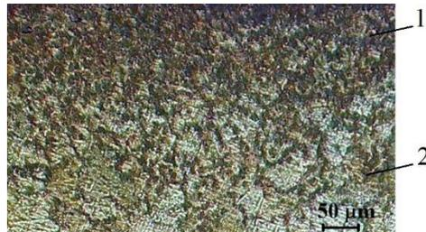
**Figure 12.** Structure of the near-surface layer of the L62 copper-zinc alloy after laser treatment. Etched section, the surface of which is located at an angle of about  $5^\circ$  to the treated surface. At such an angle of inclination, the size of studied section on the image increased by 11.4 times. 1—near-surface layer; 2—structure of the material without pores.
