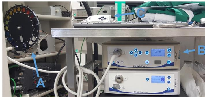
**Figure 2.** Stereo-spectral system setup: (A) the Xe light source with the filter-wheel, (B) the capturing unit, and (C) the endoscopic head.
