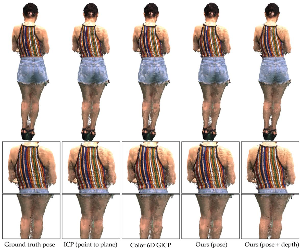
**Figure 13.** Point cloud rendering results. **First row:** Merged point clouds. **Second row:** Magnified regions in which our depth refinement algorithm produces improved results. **Third row:** Magnified regions in which our depth refinement algorithm produces artifacts. We note that no postprocessing method has been applied to the results.
