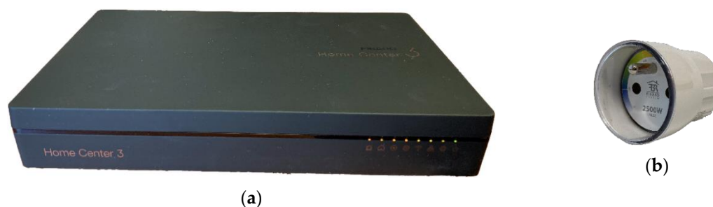
Figure 6. Fibaro system: (a) Gateway for Fibaro system management—Home Center 3; (b) Fibaro Wall Plug.
