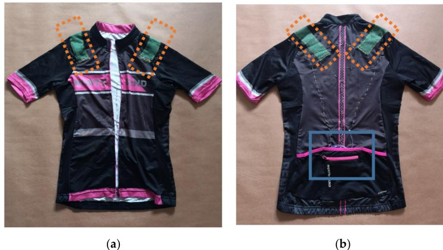
**Figure 2.** The Double Aid (DAid) smart shirt system ((a) front and (b) back) with a textile stretch sensor on each shoulder (marked by the dashed lines); the pocket on the back (marked by the blue line) is used for the data acquisition module.
