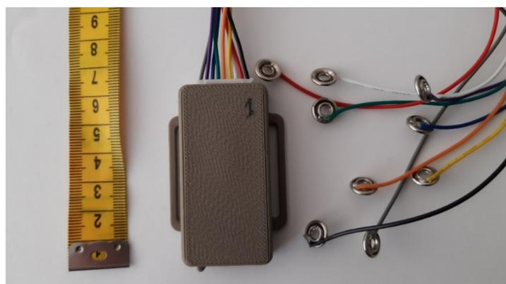
**Figure 3.** The data acquisition unit can measure up to eight channels and is connected to the system through textile snap fasteners. The unit measures only  $6.6 \text{ cm} \times 4 \text{ cm} \times 1.3 \text{ cm}$  and is positioned in a pocket on the back, and, thus, does not bother the user.
