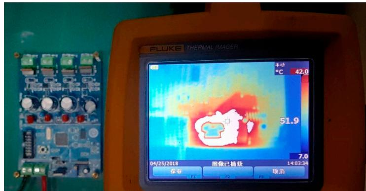
**Figure 21.** Temperature measurement result of the BU.
