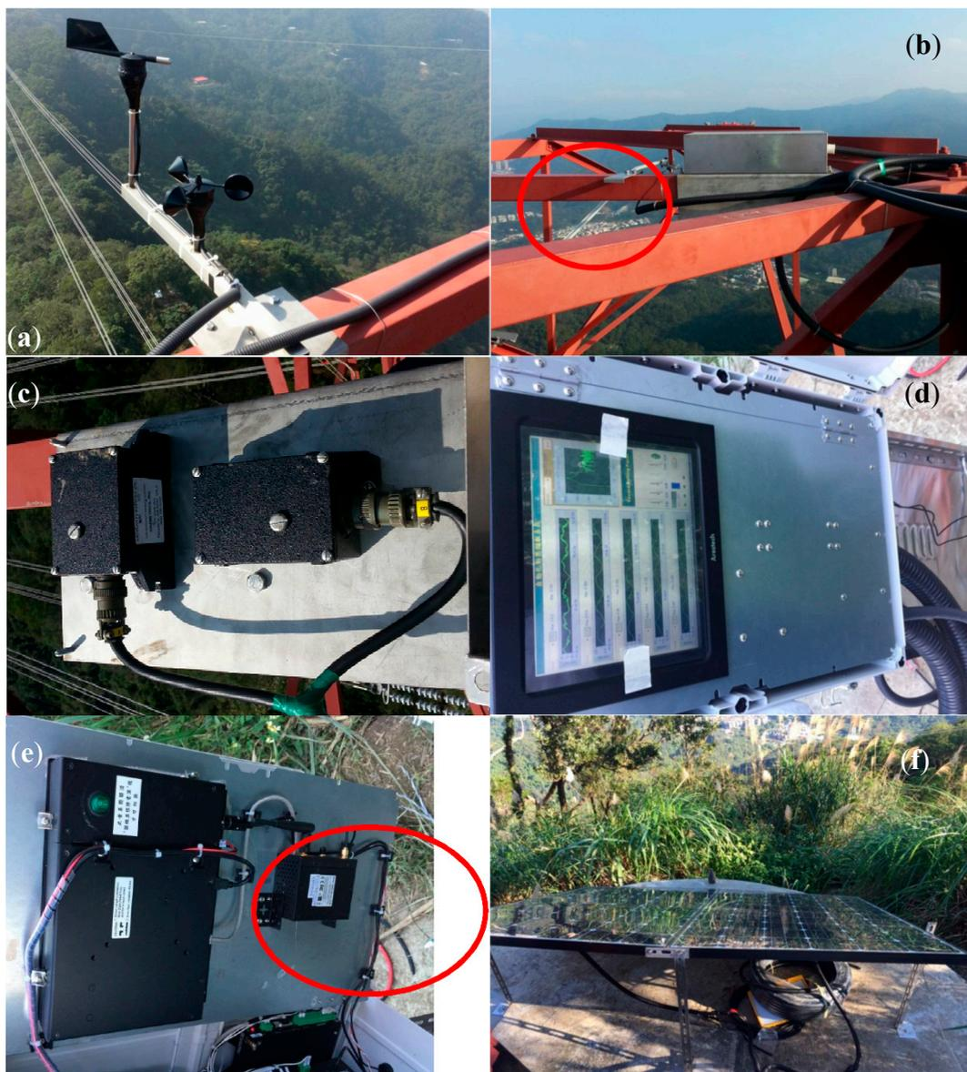
**Figure 2.** The monitoring system. (a) wind speed and wind direction sensors; (b) temperature sensor mounted on the component of PTT; (c) accelerometers; (d) data acquisition system with a monitor; (e) 4G wireless router; (f) system power set.
