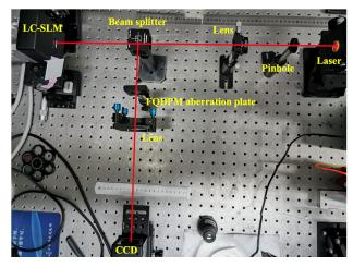
Figure 7. Schematic diagram of a real optical path.
