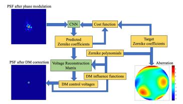
Figure 2. Working principle of the FQDPM-based CNN-AO.
