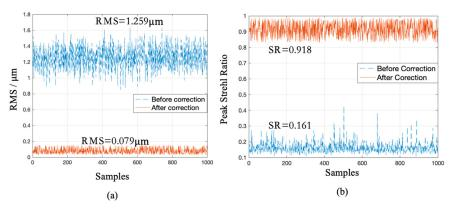
Figure 4. RMS (a) and SR (b) before and after correction of 1000 samples in the test set.
