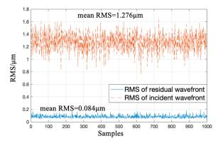
Figure 8. Wavefront reconstruction accuracy of samples in the test set.
