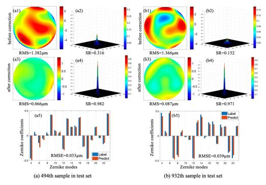
Figure 5. Correction results of 494th (a) and 932nd (b) samples in test set.
