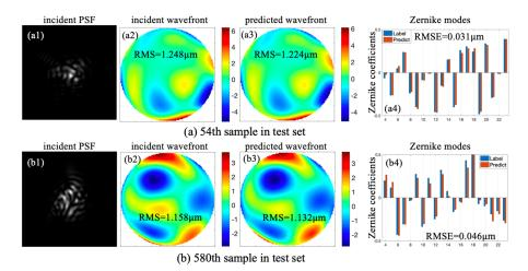
Figure 9. Reconstruction results of 54th (a) and 580th (b) samples in the test set.
