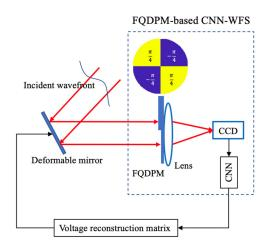
**Figure 1.** Schematic diagram of the four-quadrant discrete phase modulation (FQDPM)-based convolutional neural network adaptive optics (CNN-AO) system.
