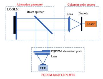
Figure 6. Schematic diagram of the optical system structure.
