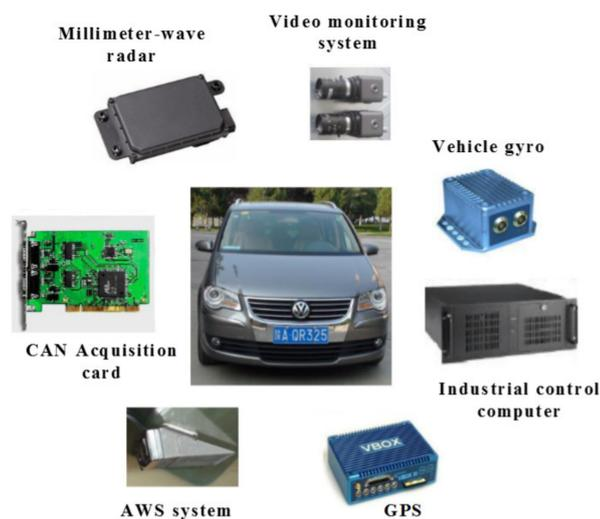
**Figure 5.** The test vehicle and related equipment.
