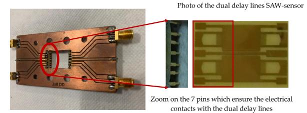
Photo of the PCB with 4 SMA connectors
