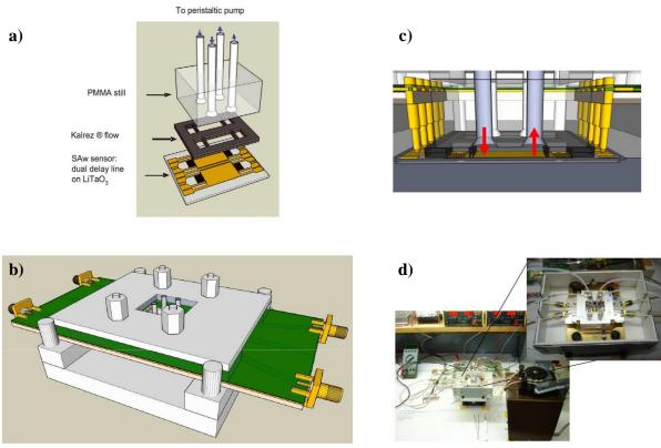
Figure S4. Details of the fluidic system
