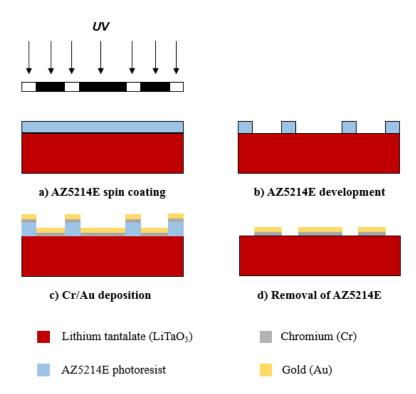
Figure S1. Manufacturing process of SAW devices in LAUM's clean room.
