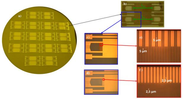
Figure S2. Photos of the SAW sensor and further details of the interdigital transducers (IDTs).
