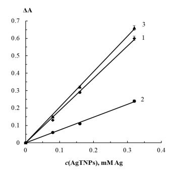
**Figure 6.** Change in the absorbance of AgTNPs solutions in the presence of 50  $\mu$ M hydrogen peroxide (1), 300  $\mu$ M *tert*-butyl hydroperoxide (2) and 3  $\mu$ M peracetic acid (3) depending on the AgTNPs concentration. pH 6, t = 20 min.
