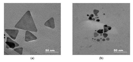
**Figure 1.** A TEM image of silver triangular nanoplates (AgTNPs) before (**a**) and after (**b**) the interaction with hydrogen peroxide. c (AgTNPs) = 0.16 mM Ag, c (HP) = 30  $\mu$ M, pH 6.
