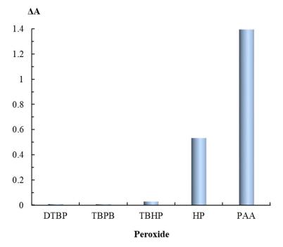
**Figure 3.** Change in the absorbance of AgTNPs solutions depending on the nature of a peroxide. c(AgTNPs) = 0.16 mM Ag, c(peroxide) = 0.1 mM, pH 6, t = 10 min.
