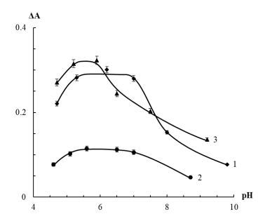
**Figure 4.** Change in the absorbance of AgTNPs solutions in the presence of hydrogen peroxide (1), *tert*-butyl hydroperoxide (2) and peracetic acid (3) depending on pH. *c* (AgTNPs) = 0.16 mM Ag; (1) *c* (HP) = 50  $\mu$ M, *t* = 10 min; (2) *c* (TBHP) = 300  $\mu$ M, *t* = 20 min; (3) *c* (PAA) = 3  $\mu$ M, *t* = 15 min.
