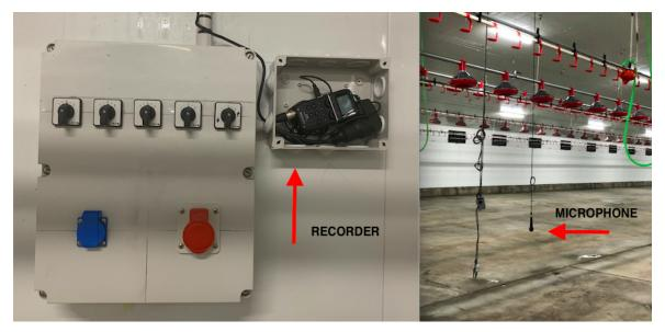
**Figure 2.** Acoustic equipment deployment in the farm H1. On the left, the recorder location. On the right, the microphone hanging from the ceiling in order to avoid physical interaction with the birds.
