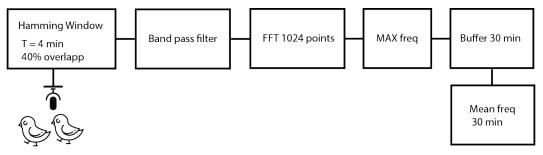
Figure 4. Peak frequency detection algorithm implementation.
