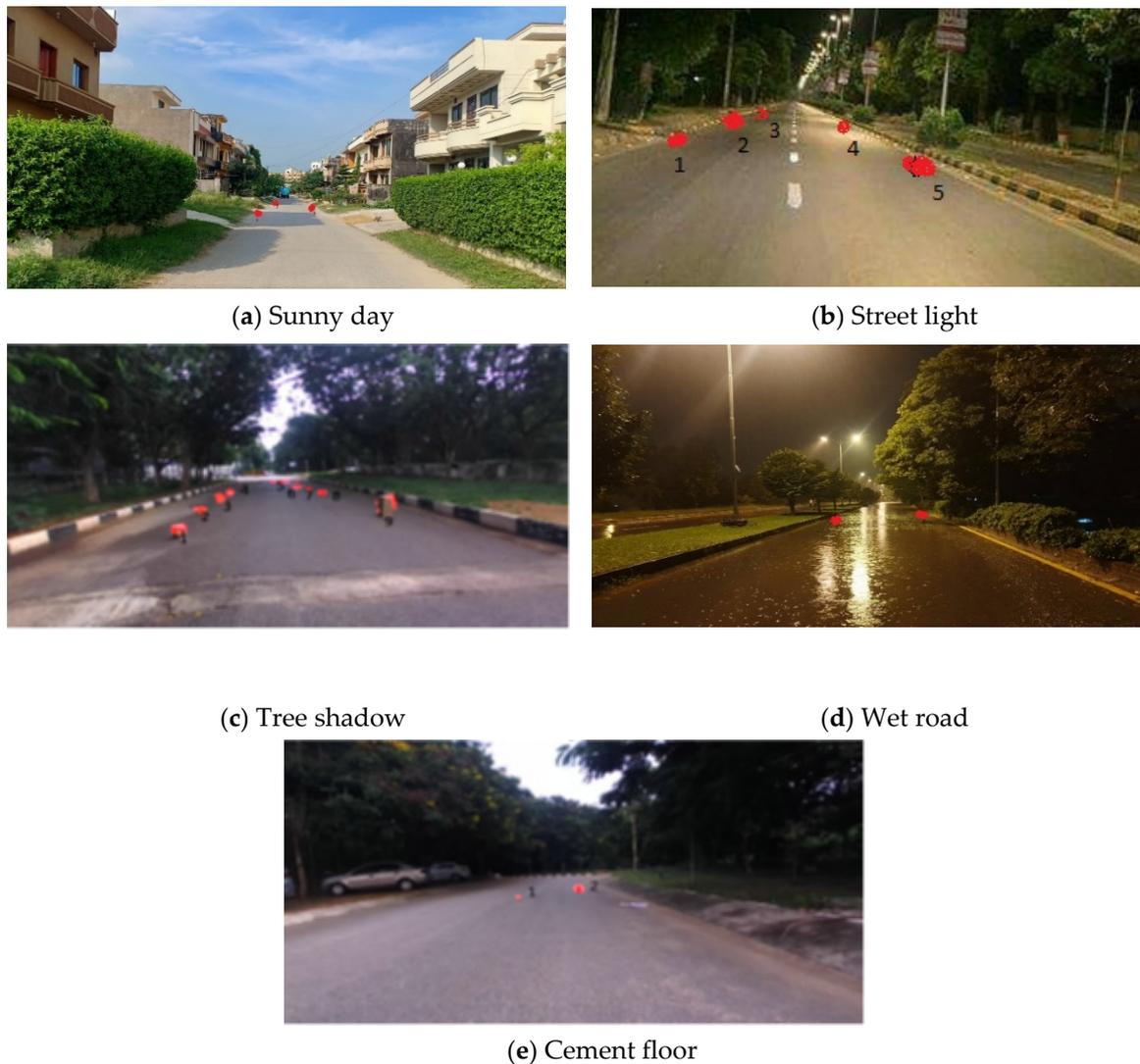
**Figure 7.** Obstacles in the captured image successfully identified by Markov random field (MRF) model.
