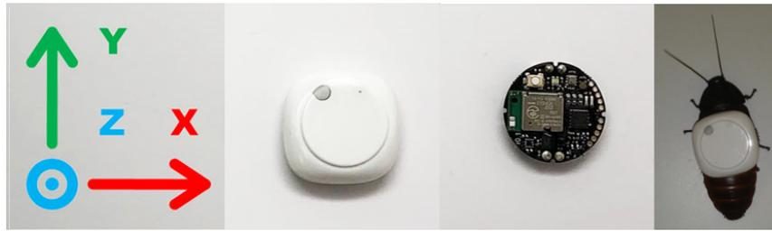
**Figure 7.** MetaMotion C Sensor Board: From left to right: (1) Coordinate frame of MetaMotion C sensor board (this is the body frame of our algorithm); (2) 3D-printed MetaMotion C case; (3) MetaMotion C PCB; (4) The IMU (inside the case) is mounted to the thorax of the biobot with the +Y direction of the IMU facing in the direction of the biobot’s antennae.
