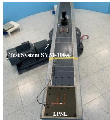
**Figure 17.** Experimental setup of overload tests.
