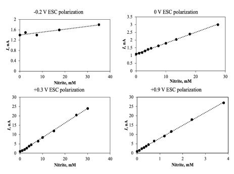
**Figure 6.** Calibration curves of a  $NO_2^-$  biosensor polarized at various ESC potentials. A potentiostat as shown in Figure 5 was not applied for this experiment, but the calibration curves were still linear, indicating that the current in the ESC circuit was constant during the recording of each calibration curve that required about 1 h. (data obtained from the laboratory of the authors).
