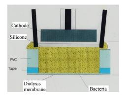
**Figure 2.** Design of a macroscale biosensor where the bacteria are housed in a 0.3–0.5 mm diameter hole drilled in a PVC or PET plate. (Original image from authors).
