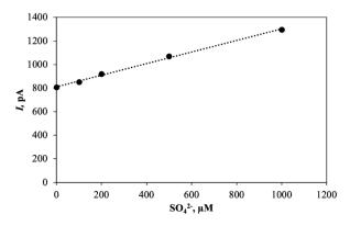
**Figure 7.** Calibration curve for  $SO_4^{2-}$  biosensor with 70 um tip. The 90% response time was 5 min due to a long diffusion path through a 400 µm layer of bacterial biomass. (Data was obtained from the laboratory of the presented authors).
