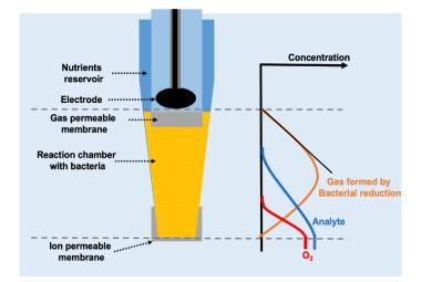
**Figure 1.** Schematic representation of biosensor based on bacteria respiring and thus reducing an electron acceptor such as  $NO_2^-$  to a gas (in this case  $N_2O$ ) that can be detected by an amperometric Clark-type gas sensor. Such sensors have been realized fore  $NO_2^-$ ,  $NO_x^-$  (i.e.,  $NO_3^- + NO_2^-$ ) and for  $SO_4^{2-}$  that is reduced to  $H_2S$ . (Original image from authors).
