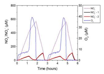
**Figure 3.** Cycles of  $O_2$ ,  $NO_x^-$  and  $NO_2^-$  in a pilot-scale wastewater treatment plant exposed to aeration cycles.  $NO_x^-$  rose upon start of aeration and decreased when aeration was stopped. Nitrite exhibited a more complex dependence of aeration/anoxia reflecting balance between  $NO_2^-$  producing and comsuming processes. Shown are traces from two  $NO_2^-$  sensors showing almost identical results. (Data was obtained from the laboratory of the presented authors).
