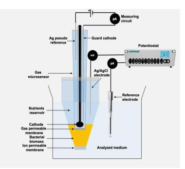
**Figure 5.** Schematic representation of the ESC technique where a potentiostat is used to assure a constant current between the Ag/AgCl electrode in the nutrient reservoir of the biosensor and an external reference. (Original image from authors).
