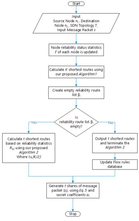
Figure 2. Flow chart for the mechanism of Obfuscation of routing paths in IoT-SDN.
