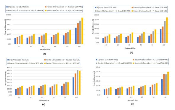
**Figure 7.** Average execution time of our route obfuscation algorithm. (a) Load = 200 MB; (b) Load = 300 MB; (c) Load = 400 MB; (d) Load = 500 MB.
