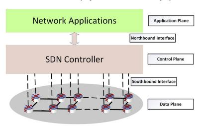
Figure 1. Software-defined network (SDN) architecture.
