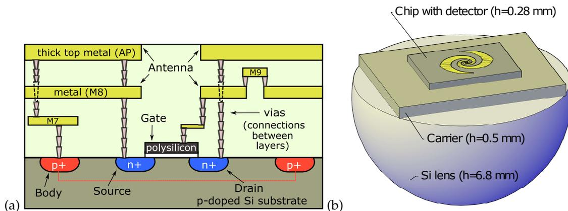
**Figure 1.** (a) Schematic cross-sectional view of the detector chip (not to scale); (b) Device with the monolithically integrated log-spiral antenna mounted on a carrier substrate and placed on a hyper-hemispherical lens (diameter of the spherical part of the lens: 12 mm).
