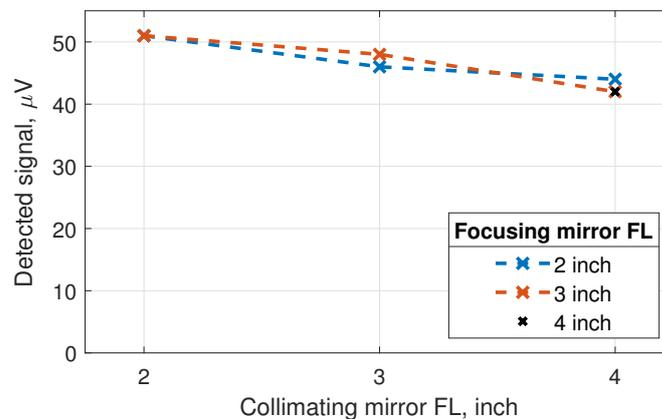
**Figure 5.** Detected signal for various combinations of paraboloidal mirrors  $M_1$  and  $M_2$  with different focal lengths (FLs); for the set-up, see Figure 4. The optimization of the configuration for the best radiation coupling was performed with the electrically chopped ceramic radiator.
