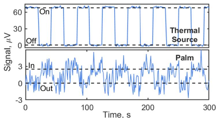
**Figure 6.** Detection of the radiation from the ceramic thermal source (top) and a human palm (bottom). In both cases, the radiation is mechanically chopped for lock-in detection. On/Off (In/Out) modulation at 25 mHz (period of 40 s). The signal-to-noise ratio (SNR) is 54 for the ceramic source, and 1.97 for the palm. The noise-equivalent temperature difference (NETD) for the latter amounts to 4.4 K.
