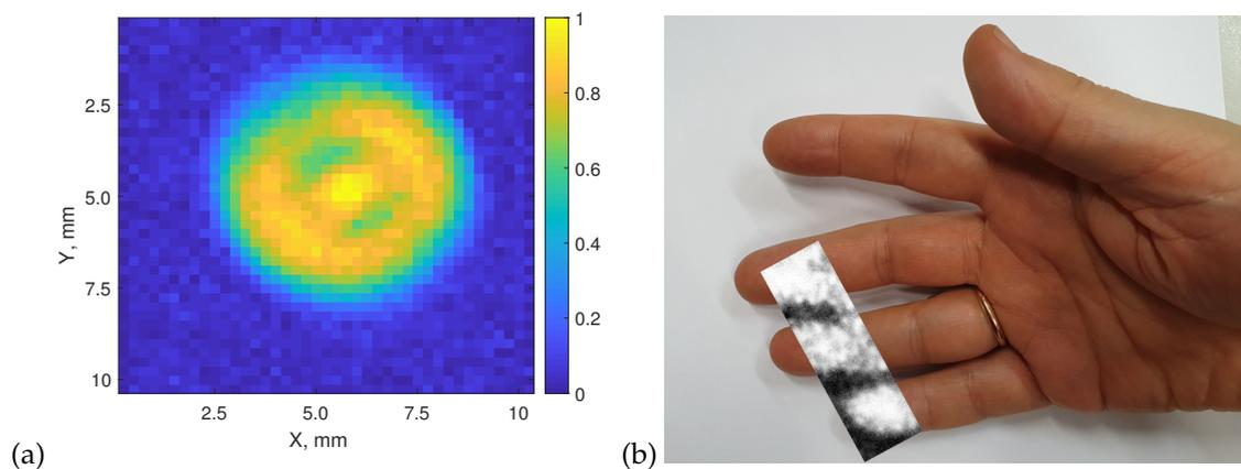
**Figure 8.** Thermal images recorded with the broadband Si CMOS TeraFET detector at room temperature. (a) image of the thermal emission pattern of the heated ceramic source; (b) image of sections of three fingers of a human hand. The image is superimposed on a photograph of the hand. In both cases, mechanical chopping of the thermal radiation was applied.
