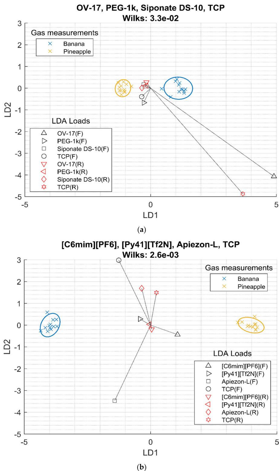
**Figure 5.** LDA bi-plot for the best sensor array using frequency (F) and resistance (R) data of the 2 scents measured. (a) Conventional films. (b) Best sensing film selection.
