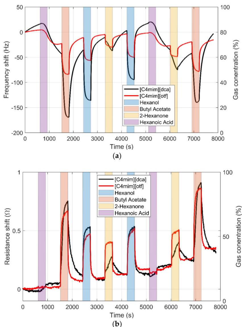
**Figure 1.** (a) Typical response of the sensors [C4mim][dca] and [C4mim][otf]. (b) Frequency response to the four VOCs. Resistance response to the four VOCs at maximum concentration.
