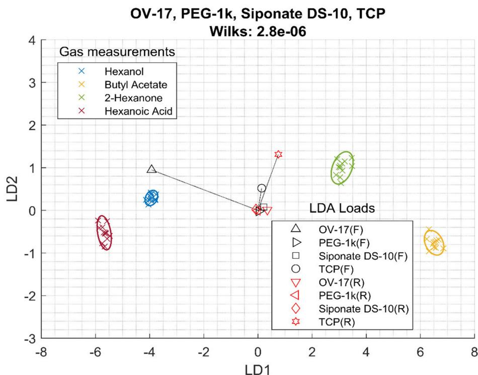
**Figure 3.** LDA of array of four best conventional films using frequency (F) and resistance (R) data.
