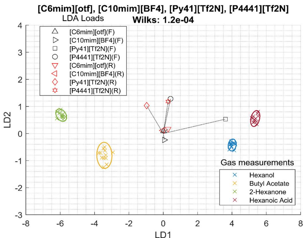
**Figure 2.** Linear discrimination analysis (LDA) of measurements of room temperature ionic liquids (RTILs) regarding the frequency (F) and resistance (R) data.
