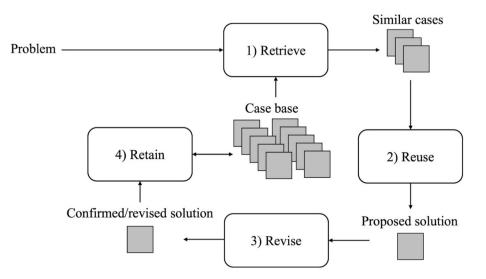
Figure 3. Schematic representation of the CBR cycle proposed by Aamodt and Plaza [43].
