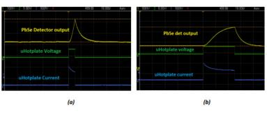
**Figure 13.** (**a**) System output with hotplate pulsed at 5 ms and (**b**) System output with hotplate pulsed at 25 ms.
