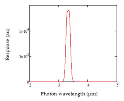
Figure 11. Source–Detector–Filter product for methane gas detection.
