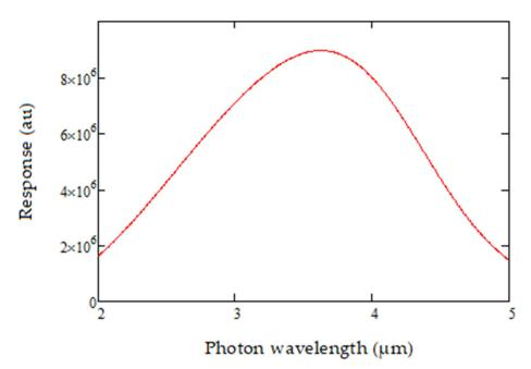
Figure 8. Source-Detector product over the detection range of interest.
