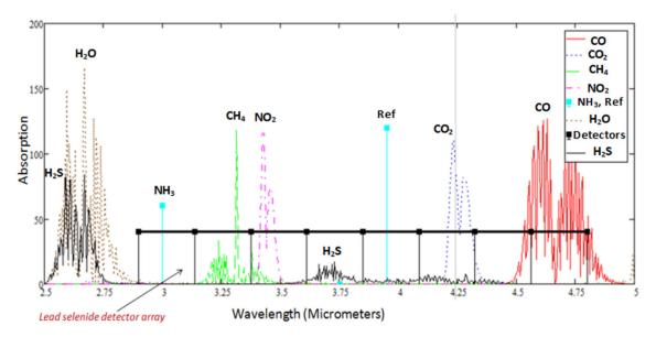
Figure 3. Lead selenide detector alignment with gas absorption spectra.
