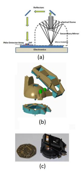
**Figure 1.** (a) Schematic of the multi-gas sensor optics; (b) exploded view of the three-piece optical assembly; (c) assembled injection moulded optics (UK 50 pence piece shown for scale—23 mm diameter).
