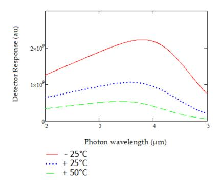
Figure 7. Lead selenide detector response modelled at different temperatures in the 2 to 5 μm range.
