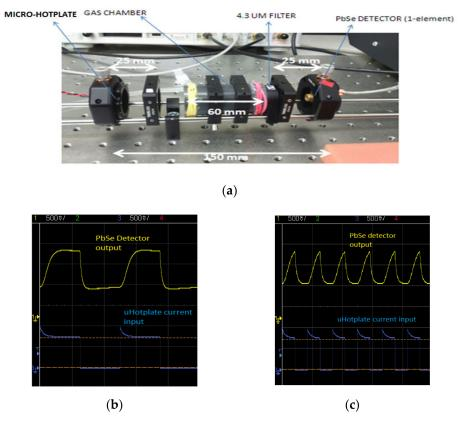
**Figure 4.** (a) Demonstrator setup for gas detection with 25 mm optical lenses, (b) output with the hotplate driven with a 4 Hz square wave, and (c) output with hotplate driven with 12 Hz square wave.
