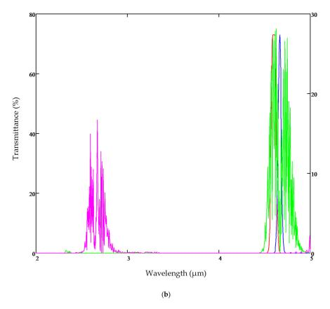
**Figure 16.** (a) Design A: CO filter transmission using 480 nm wide commercially available signal [37] and reference filters. (b) CO filter transmission using 100 nm wide in-house designed signal filter and reference filters [33].
