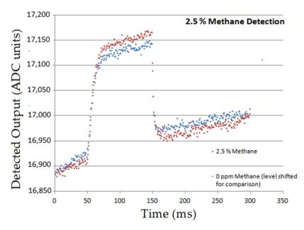
Figure 15. PbSe detector output demonstrating 2.5% Methane detection.
