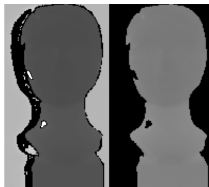
Figure 8. Input depth image with interference. The left image with extreme interference regions before depth thresholding. The right image without extreme interference regions after depth thresholding.
